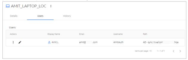
If a user is currently blocked from accessing the workstation due to enforcement of push fatigue protection mechanisms [32], the icon appears in the row of the user. To manually unblock the user, click and select **Unblock Device For User**.
