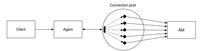
When a client makes a request, the agent intercepts the request, and uses the connection pool to connect to AM. If a connection is available, the agent uses that connection. The client is unaware of the connection reuse.
