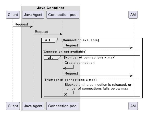
When <u>Enable Connection Pooling</u> is true, use the following properties to tune the connection pool:
